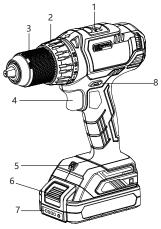
1.Speed Selector button 2.Torque Presettina Rina 5.LED Light 6.Battery Pack
