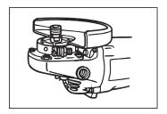
• Installing or Removing Depressed Center Wheel Screw the inner flange onto the spindle, then put the wheel into the spindle and install it on the inner flange, and screw the outer flange to the spindle. Press the spindle lock device to prevent the spindle from rotating. Then use the lock nut wrench to tighten the outer flange.
