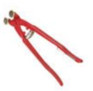
• Specially for cutting narrow strips of a maximum of 7/16" (1 cm). Equipped with tungsten carbide GOLD scoring wheels with titanium surface treatment for longer useful life. By means of a gentle turn, the wheels can be repositioned when their vertex starts getting worn. If totally worn, they can be replaced using their corresponding spare piece, 0 3/4" (18 mm) GOLD spare scoring wheel long-life (Ref.01953).
