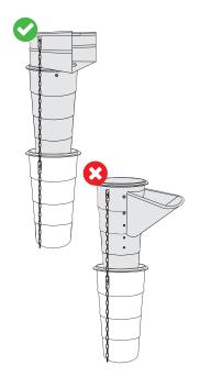
TOP HOPPER DO NOT start the column with a side hopper piece. Unsecured, loose or unscrewed hopper section
