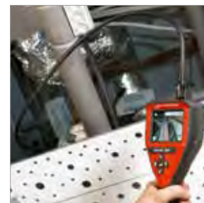
Camera head with high-performance LEDs
