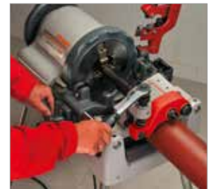
Cost-effective production of grooves
