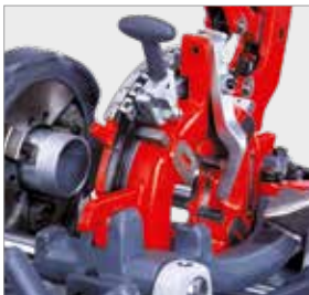
Automatic die head with integrated oil supply
