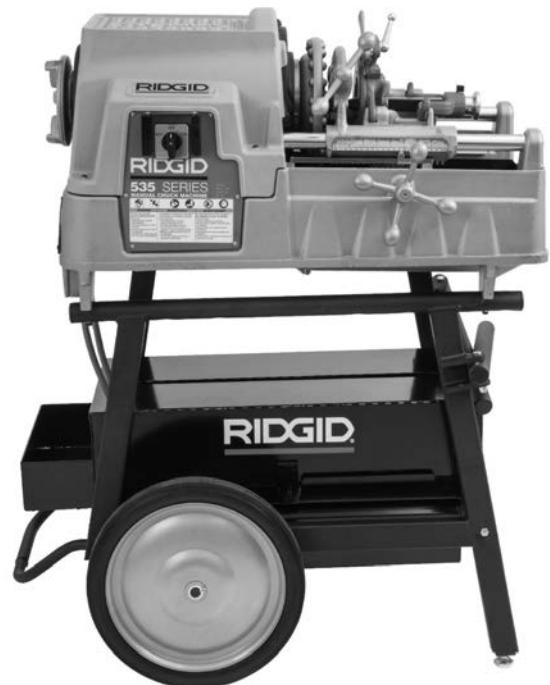
Figure 28 – Machine prepared for Transport
