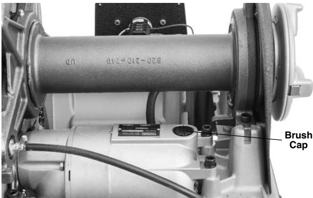
Figure 34 – Removing Motor Cover/Changing Brushes
