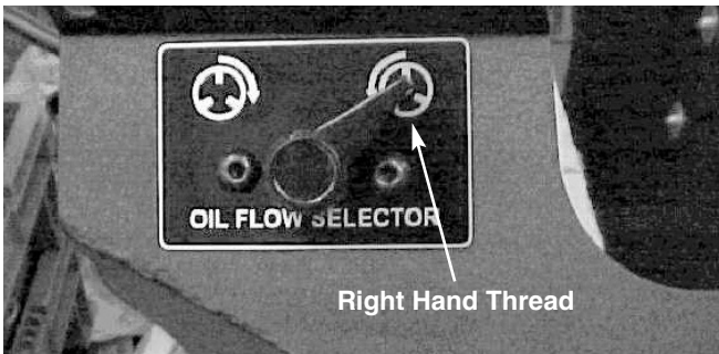
Figure 24 – LH or RH Oil Flow Selector
