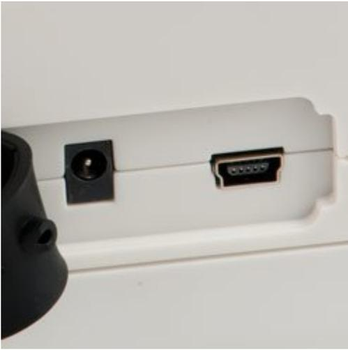
Here you can see the inputs at the colourimeter PCE-CSM 2 and PCE-CSM 4. One of these is compatible with the adapter for recharging the device's battery (in image left input). The other one is a RS232 interface for USB connections to a computer or printer, in order to evaluate the data by means of the software included in delivery.
