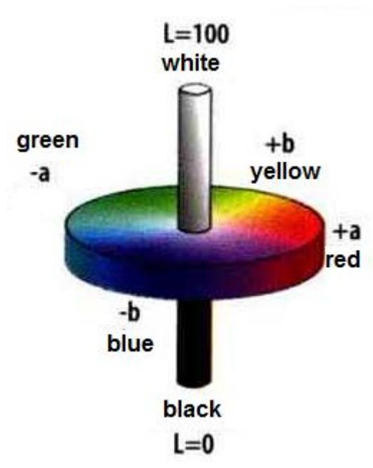
Here you can see the colour space L\*a\*b. This colour space covers all colors that are visible with the naked eye. L=100 stands for white and L=0 for black. "a+" and "a-" or "b+" and "b-" stands for the colour contrasts red, green, yellow and blue.
