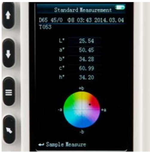
Here you can see the user interface of the Colorimeter PCE-CSM 2 and PCE-CSM 4 during standard measurements. That interface starts as soon as the device initiates the measuring process. The Colorimeter does not only display the various values of the parameter, but it also illustrates the measuring results in a graphic as you can see here.
