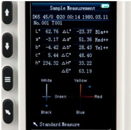
After performing the measurement you can also enter the sampling mode. Here the relevant parameters are displayed in detail. They are also visualized by two graphics for all the colours and for black and white. Furthermore the Colorimeter PCE-CSM 2 and PCE-CSM 4 thus offers a precise overview for all kinds of measurements.
