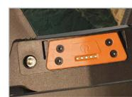
**Battery Level Indication on battery** pack va 5 LED battery level indicator. Each Led indicates 20% charge
