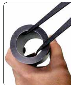
Inside Caliper in use to measure the internal diameter of a cylinder
