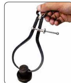
Outside Caliper being used to inspect the external diameter of a machined component
